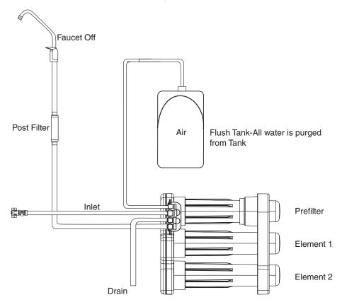
Low TDS water has flushed out the inlet side of the elements. Complete process may take 3 to 8 minutes.
