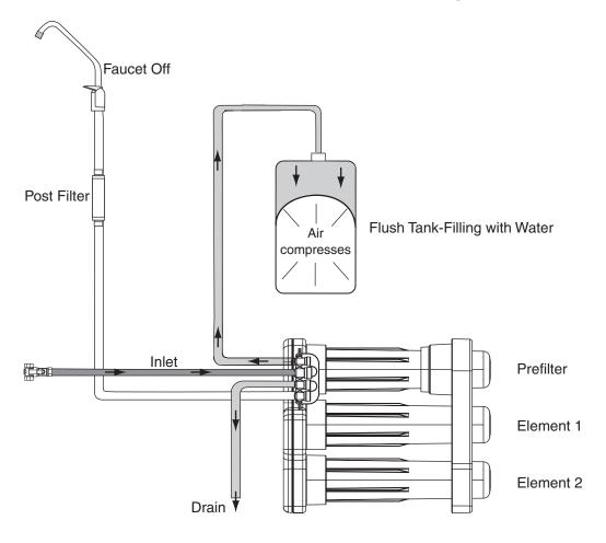
Merlin System is Producing Permeate Water for Flush
