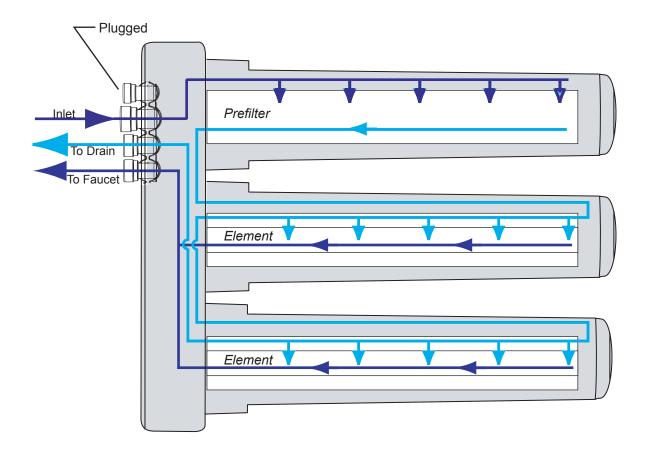
Figure 9 The Merlin Flow Pattern
