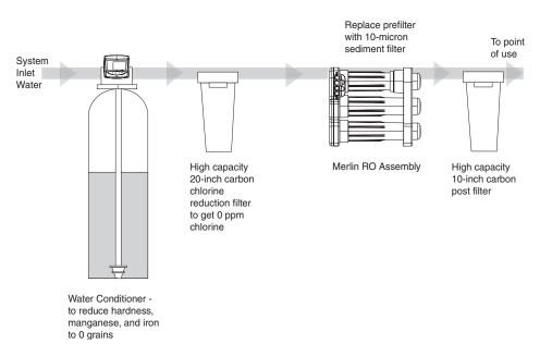
Figure 19 - 20 to 100 Gallons (75.7 to 378 Liter) Per Day Permeate Water Use
